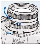
While aligning the two alignment dots (1 & 2), insert lens into the camera body. Then twist lens clockwise until it clicks and locks into place.
